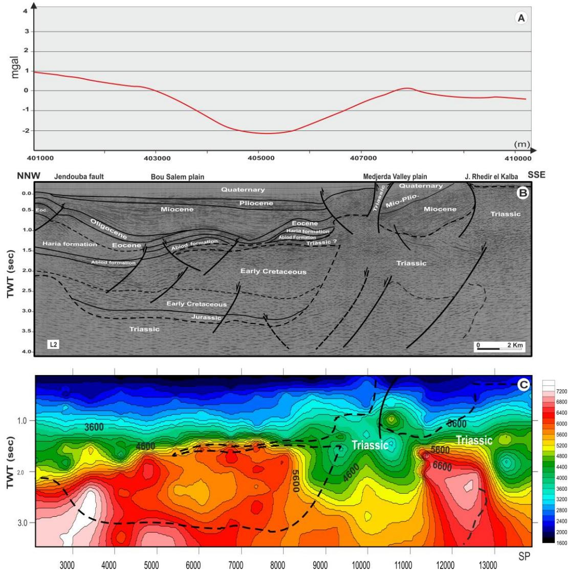
Figure 9A) Residual gravity anomaly section, B) Interpreted seismic line (L2) of the Medjerda Valley Plain domain, C) Interval velocity section of the seismic line (L2).
