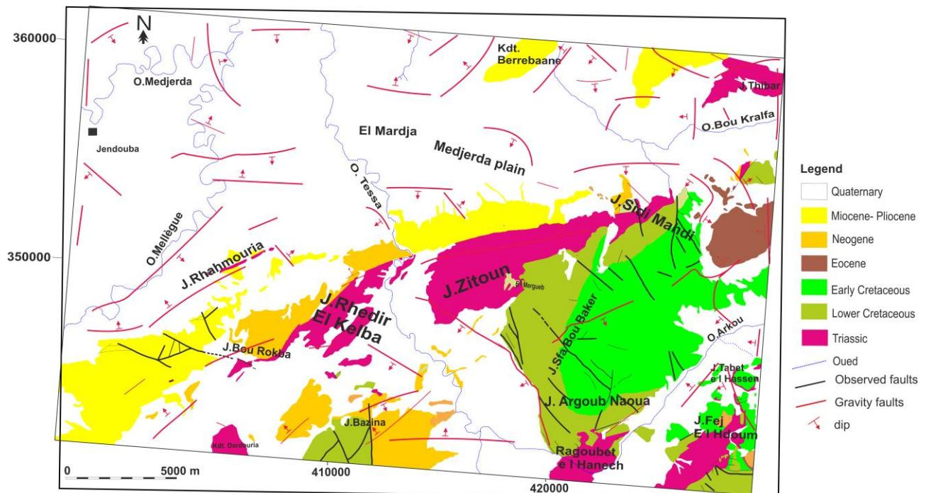
*Figure 7) Gravity lineaments map superimposed the geological map of the study area.*
