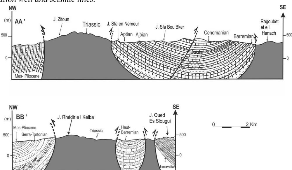
Figure 2) Geological cross-section in the study area (J. Zitoun area) showing the relation between Triassic materiel and its surrounding series.
