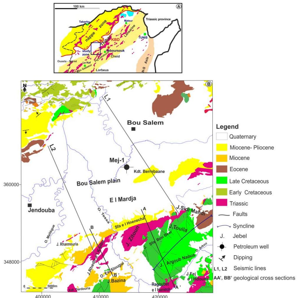
Figure 1A) Map of location of study area and salt extrusions in Northern Tunisia, B) Geological map of Triassic outcrops in the study area [after Ben Hadj et al., 1993], (J.) = Jebel. This map shows the position of used exploration well and seismic lines.
