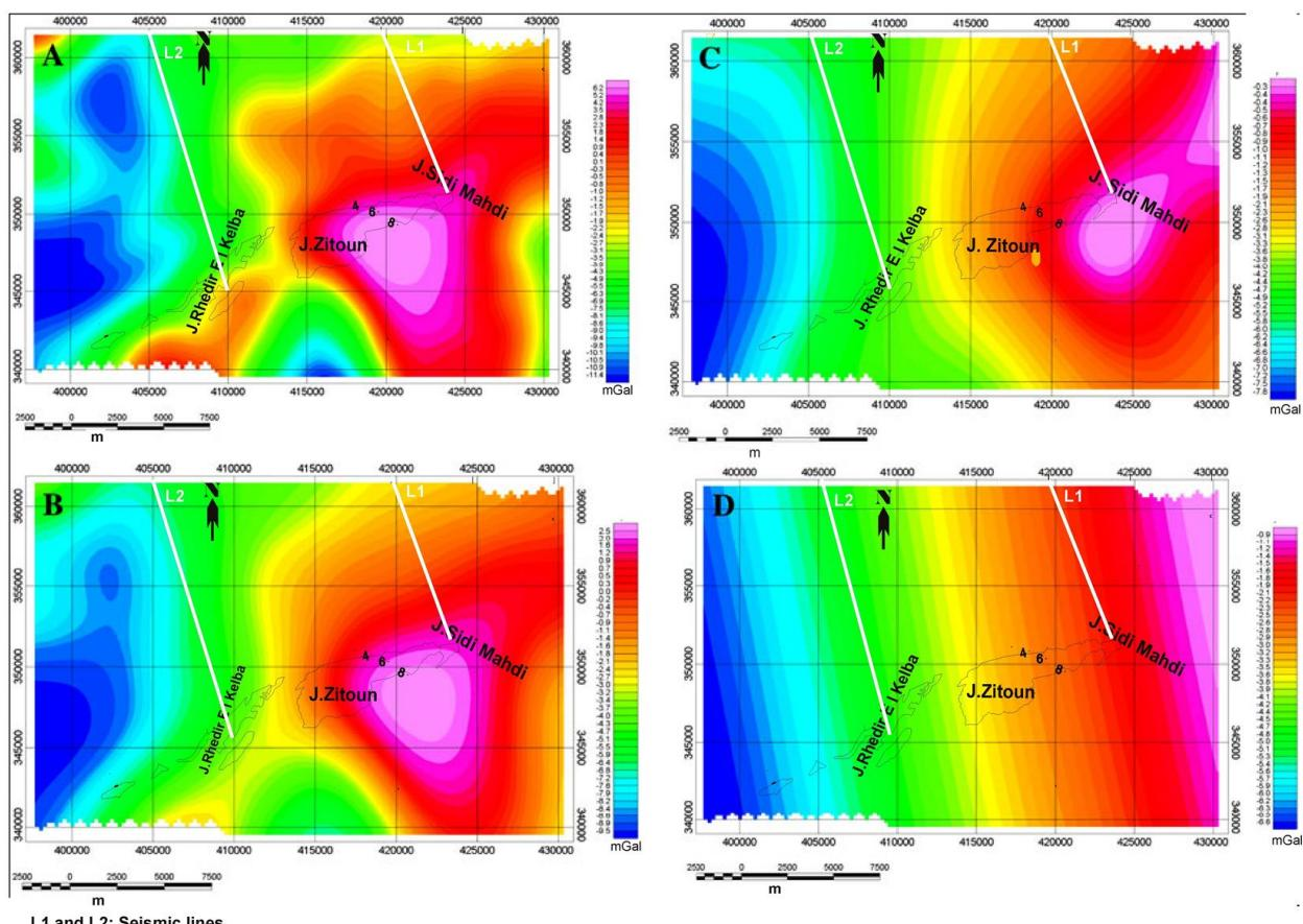
Figure 4) Upward continuation maps showing a regional gravity field: A- 1000 m, B- 5000 m, C- 10000 m, D- 27000 m.
