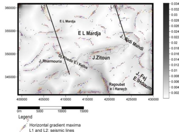
*Figure 6) Maxima of the horizontal gradient of the Bouguer anomaly and their extended upwards at different altitudes illustrating the interpreted gravity lineaments: black points (0 m), red points (250 m), blue points (500 m), Yellow points (1000 m), green points (1500 m) and brown points (2000 m).*
