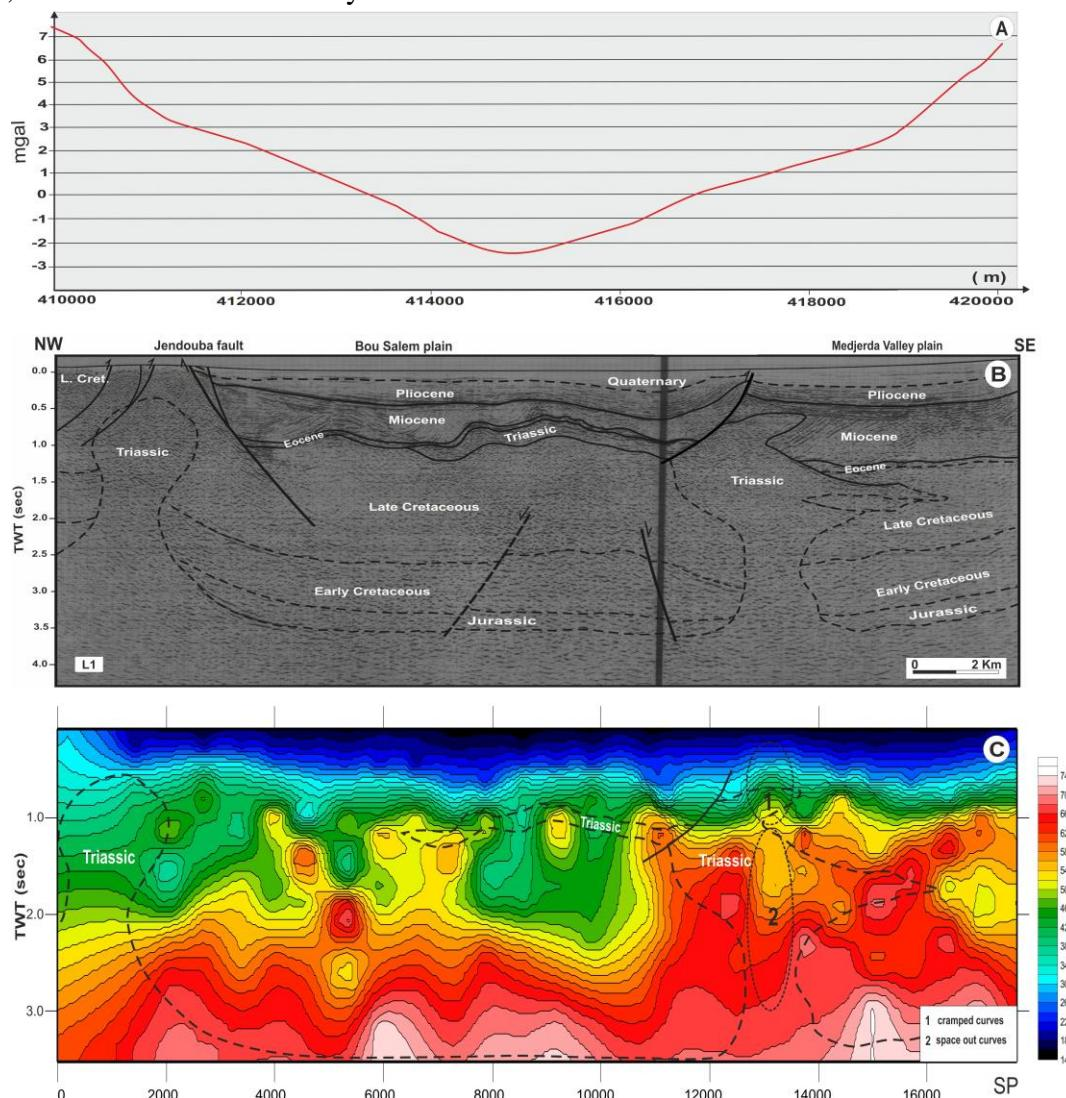
Figure 8A) Residual gravity anomaly section, B) Interpreted seismic line (L1) of the Medjerda Valley Plain domain, C) Interval velocity section of the seismic line (L1).
