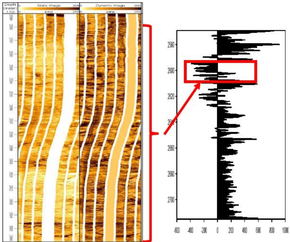
Figure 8) Display conductive zone in image log (means open fracture), and velocity deviation log indicated readings near -500 amount in conductive zone.
