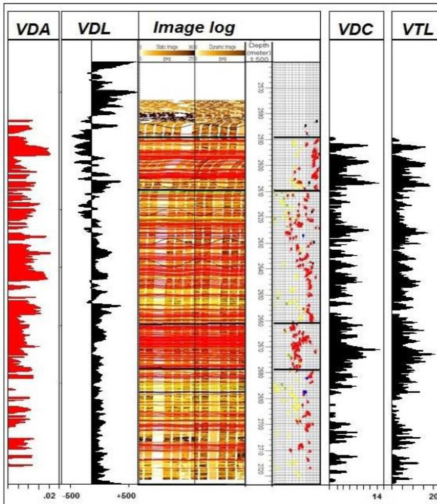
Figure 7) Velocity deviation showing a negative amount in depth of 2594 to 2610 meters and aperture fracture has a pick on this depth. Fracture length and density have two picks on 2605-2660 meters.
