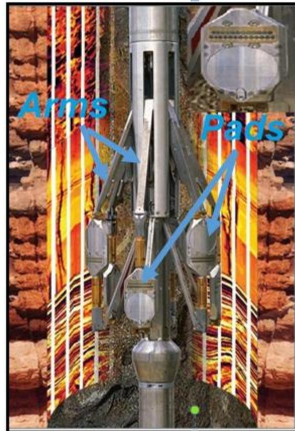
Figure 3) XRFMI tools obtain six independent arms and six pads with 25 buttons on each pad.
