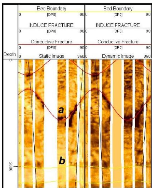
Figure 4) The Static and dynamic images from XRMI. Line- a shows a conductive feature that's seems to be open fracture, and line- b is bedding. Fractures tend to occur as linear features that generally have a dip steeper than the structural dip.
