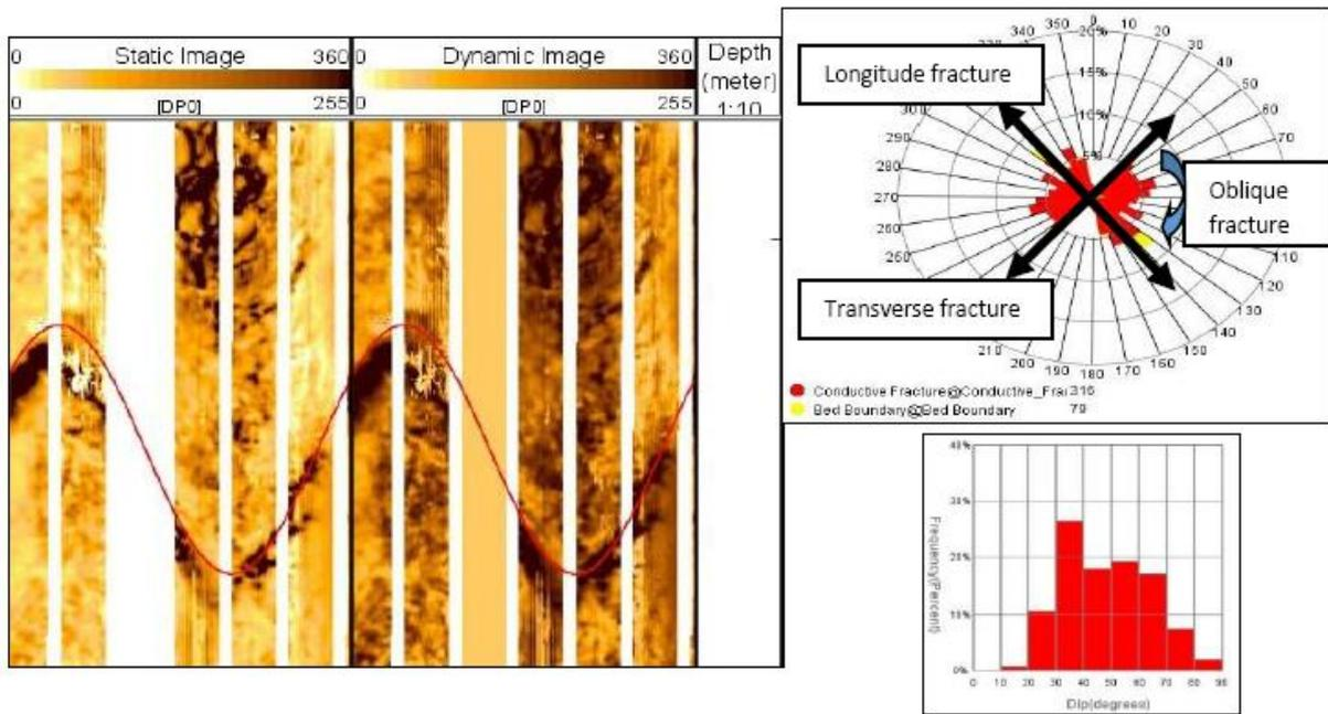
Figure 6) Display conductive zone in image log (means open fracture), and velocity deviation log indicated readings near -500 amount in conductive zone.
