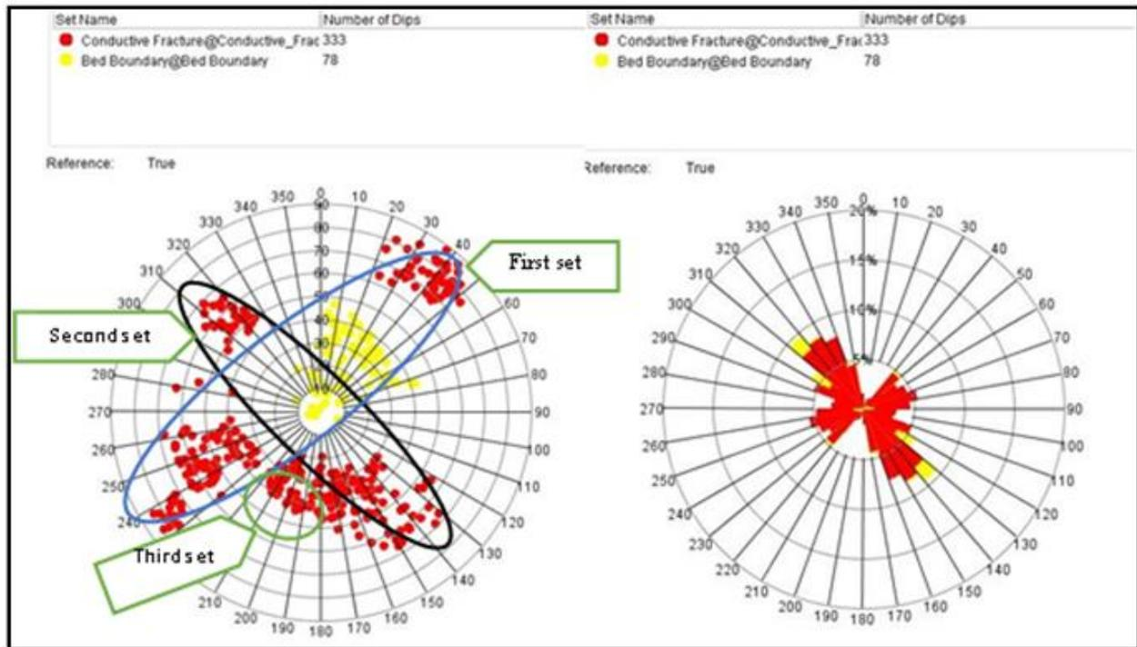
Figure 5) Result of interpreted fracture and bedding on image log, fracture (red) and bedding (yellow) stereo net and strike in well under study.
