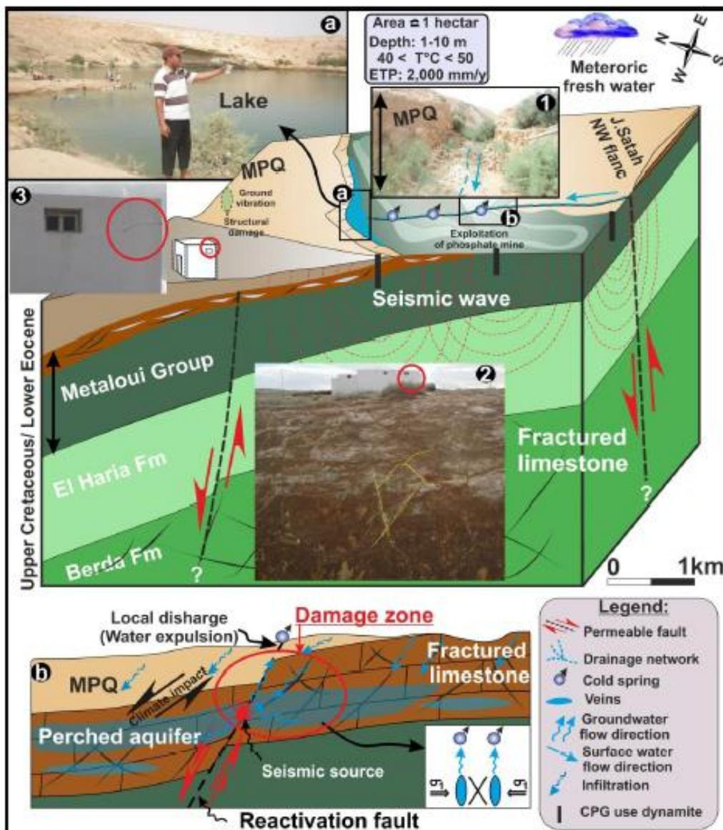
Figure 2) Conceptual model showing the hydrodynamic and the anthropogenic impact in the Gafsa mining basin.
