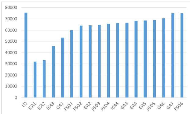
Figure 7) Volume of earthworks at different methods (M3).
