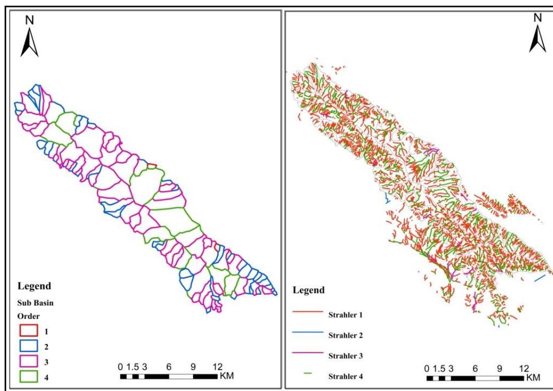
Figure 3) Drainage map of basins 1 to 4. The hydrographic network is represented according to Strahler's ordering system.
