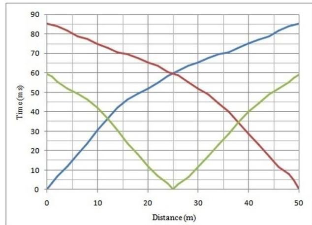
Figure 4) Time-distance curve (P waves)-Basij center
