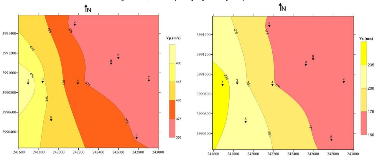
Figure 14) Velocity map up to depth of 10m.
