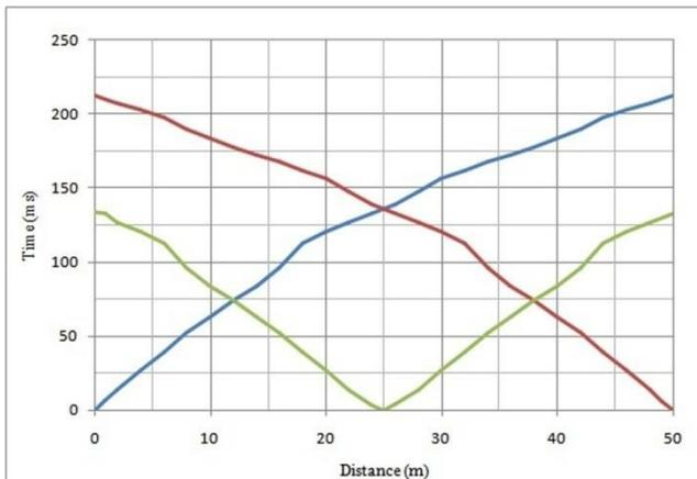
Figure 5) Time-distance curve (S waves) - Basij center
