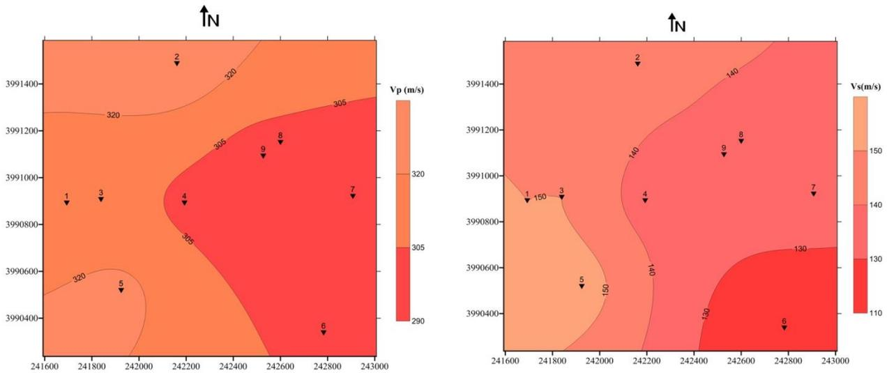
Figure 11) Velocity map up to depth of 1m.
