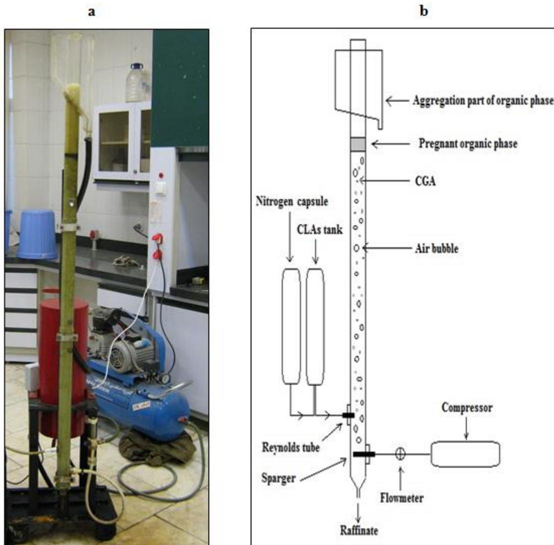
Figure 1) DNPDSSE system: a) contactor and b) schematic diagram.
