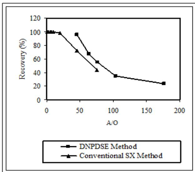
Figure 2) Recovery diagrams of the SX and DNPDSSE methods in various A/O ratios.
