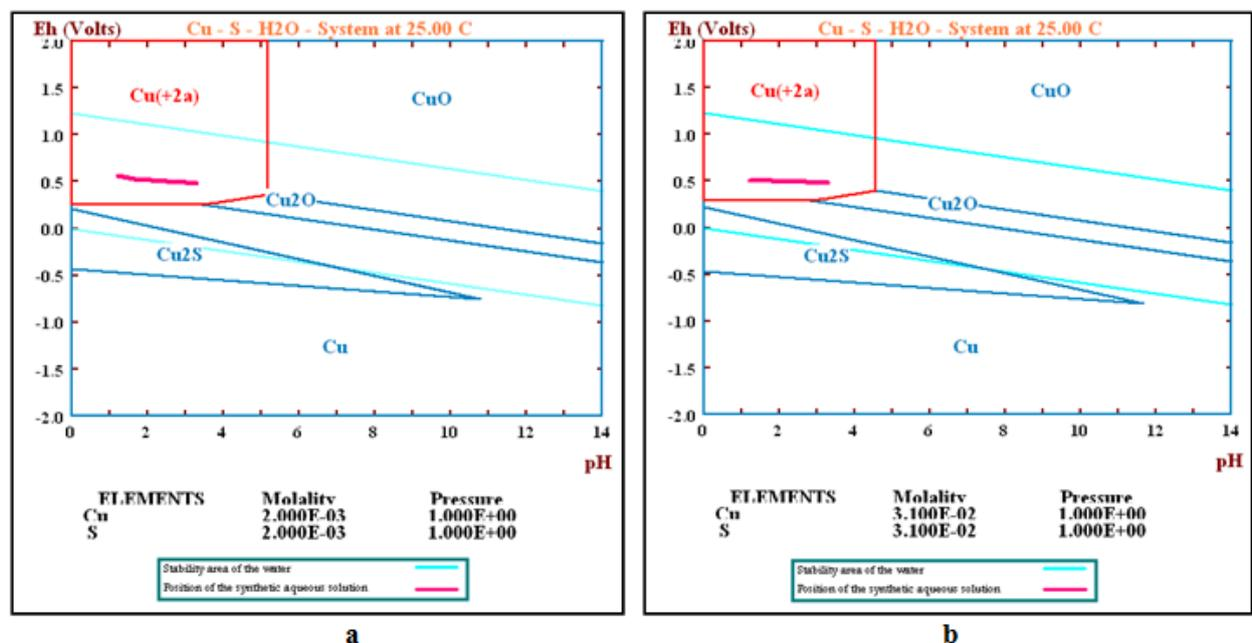
Figure 1) Eh-pH diagrams of synthetic aqueous solutions: a) dilute solution and b) dense solution.
