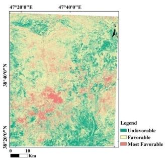
Figure 5) The categorized primary gold favorability map based on the alteration indicators derived from the FPCS method.
